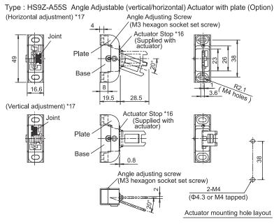
Type: HS9Z-A55 Angle Adjustable (vertical/horizontal) Actuator (Option)
