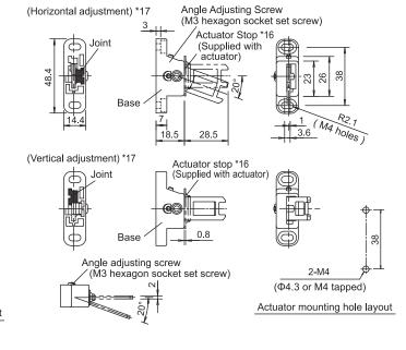
Type: HS9Z-A53 Angle Adjustable (vertical) Actuator (Option)
