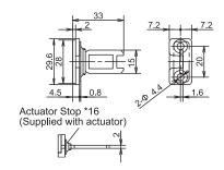
HS9Z-A51/A52 Actuator mounting hole layout
