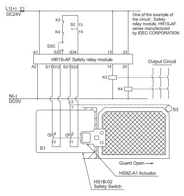
Use the monitoring device(Safety relay module) provided the capavility to detect a cross short circuit. The insulation of the cable has to withstand environmental influences. If a control device other than the one shown in the draft is used, the used control device has to be equipped with a cross short circuit monitor.
