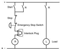
Note: When using the main circuit on AC (HS1P-1, HS1P-34), connect the emergency stop switch to Line, and the interlock plug unit to Neutral.
