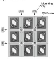
Insert the joint SLDN units into the panel cut-out from the front of the panel. Install the mounting clips as shown and tighten the screws lightly to a torque of approximately 0.39 to 0.49  $N\!\cdot\!m$ .
