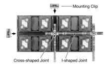
Insert the joint SLDN units into the panel cut-out from the front of the panel. Install the mounting clips as shown and tighten the screws lightly to a torque of approximately 0.39 to 0.49 N·m.
