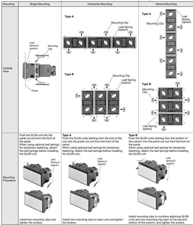
Note: Tighten the mounting clip screws to a torque of approx. 0.39 to 0.47 N·m. Leaf springs are not supplied with the SLDN unit must be ordered separately.
