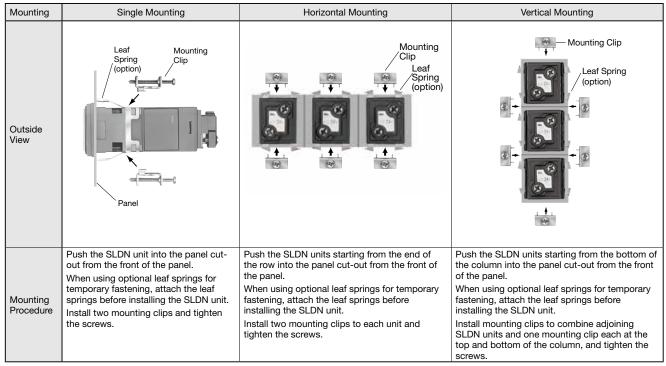
Note: Tighten the mounting clip screws to a torque of approx. 0.39 to 0.49 N·m.
