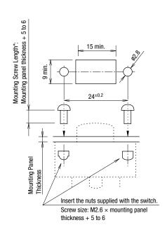
Note: When installed on a mounting panel thicker than 2 mm, the actuator surface is below the panel when the button is pressed to position 3.
